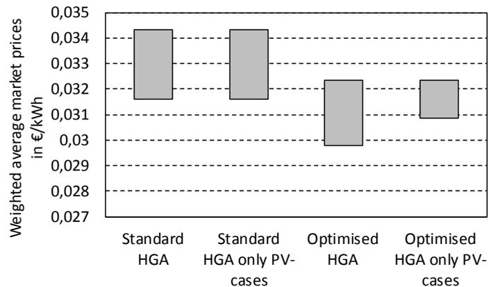
**Figure 4: Range of own-consumption rates as result of the optimised HGA operation for the FP**
