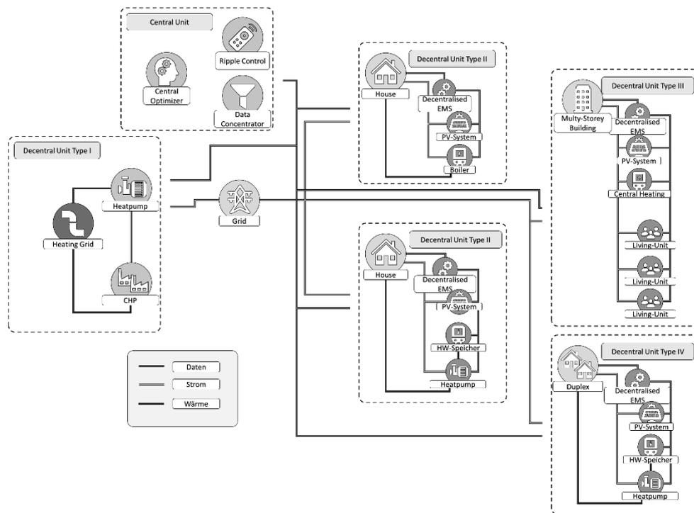
**Figure 1: Coupling of heat and electricity to create a hybrid energy system**
